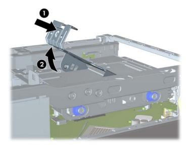
6. Lift the hard drive carrier straight up and out of the chassis.
